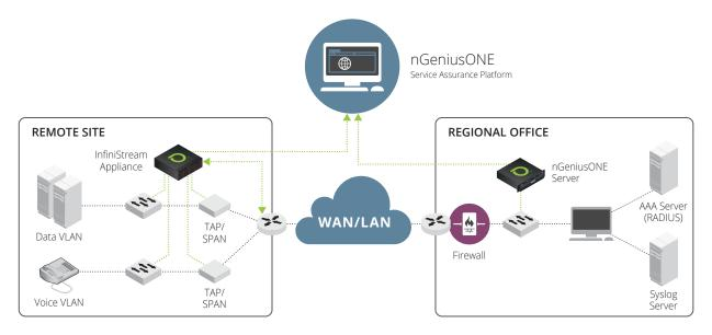
Figure 1: Tested NetScout nGeniusONE solution with the nGeniusONE platform and the InfiniStream appliance.
